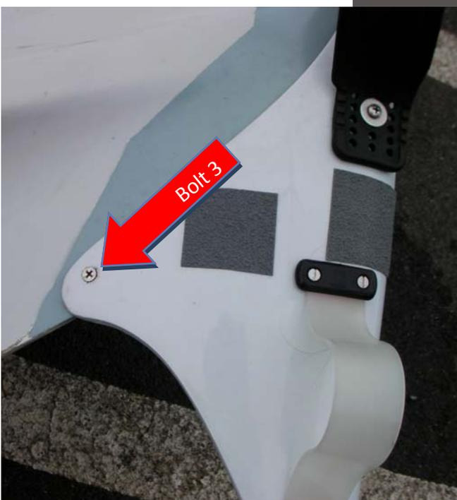
can position the third bolt again not too close to the edge of the boat or extension, ideally about 1/2 inch in from the edge.
